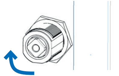
DIAGRAM 2. Fit locking nut & tighten to secure.
